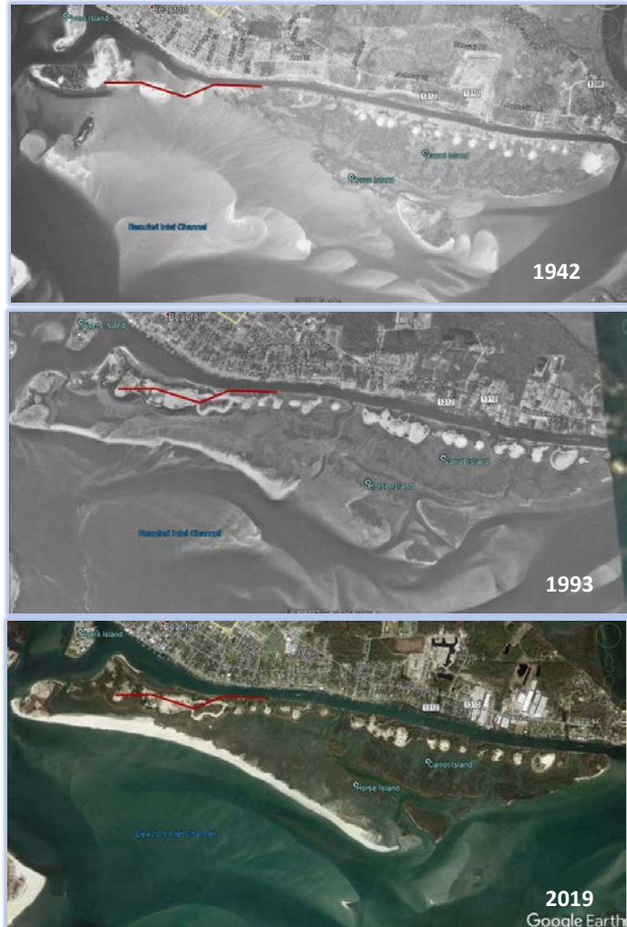
Top to bottom: 1942 (notice the rock bulkhead in red that was installed ~1915 to connect Town Marsh and Carrot Island), 1993, and 2019.
